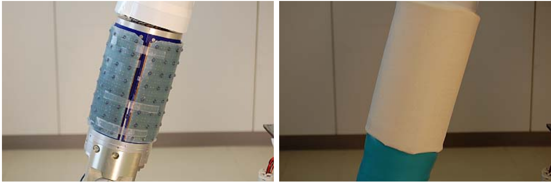
Fig. 3 Tactile sensors covering all around the arm
